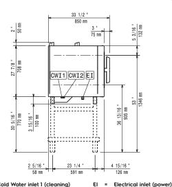
CWI1 = Cold Water inlet 1 (cleaning) CWI2 = Cold Water Inlet 2 (steam
